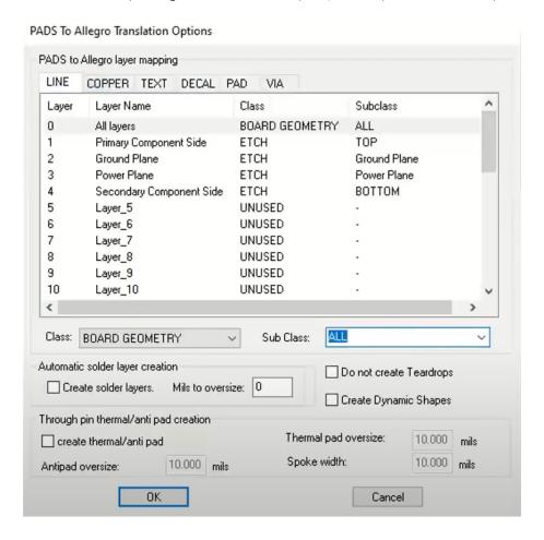
After mapping, the Command window will show the translation progress. Once the translation finishes, the translated **.BRD** file will be accessible in the folder specified in the Output Design field.
