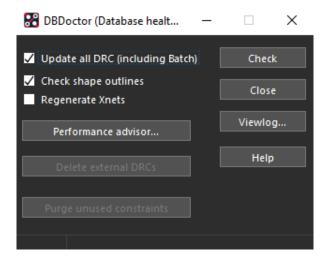
The DBDoctor will flag any errors or remaining DRC errors that should be addressed during cleanup.
